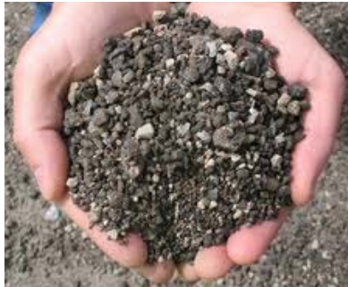
Reclaimed Asphalt Pavement
