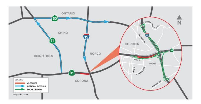
RCTC is working with Caltrans to repave lanes and repair sound walls and concrete barriers along the outer portions of eastbound and westbound 91 in Corona. Work will occur mainly between the Lincoln Avenue interchange and Interstate 15, an area with a long history of roadway settlement due to the Temescal Wash. Construction on the 91 will take place through the summer and fall, with additional weekend closures to be scheduled.
