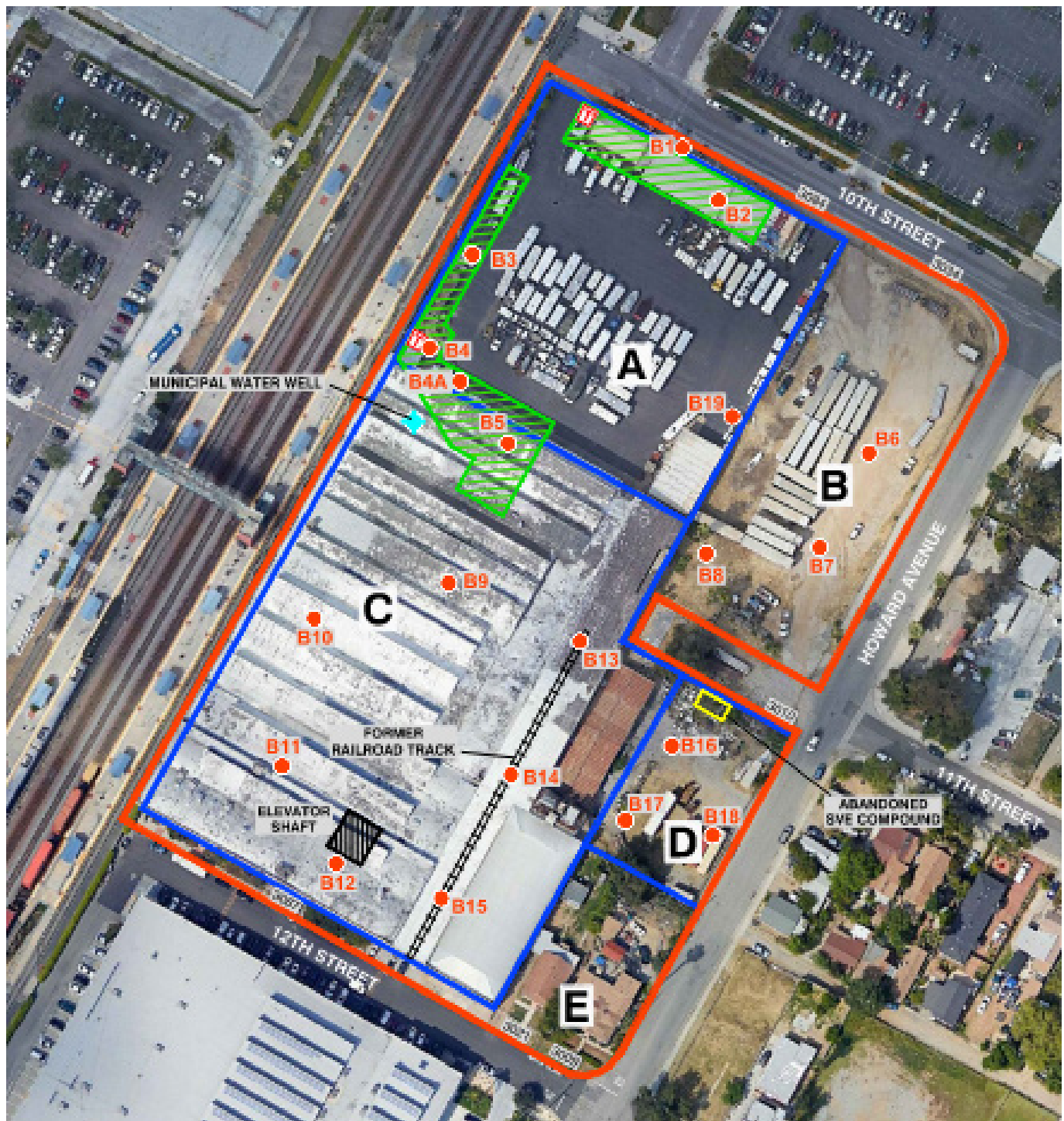
Figure 3.8-2. Limited Phase II ESA Study Area and Boring Sample Locations
